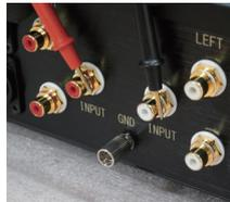
Turn on the phono equalizer and check the outer rings of the RCA inputs with a volt meter.
