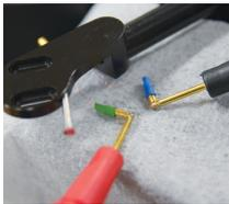
After connecting the tonearm cable to the RCA inputs, use your volt meter to check the blue and green lead cables in the tonearm headshell.
