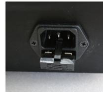
Please take out the fuse and check it as there is a possibility that the fuse is blown, missing, or of an incorrect value. Use your volt meter to confirm that the fuse has continuity. You can access the fuse by pushing out the plastic tray in the AC power supply connector on the back of the equalizer inlet.
