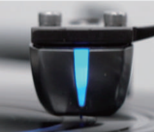
No eccentricity: Cartridge is stable
