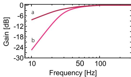
c, 50Hz switch selected OUTPUT1 output (LINE out)
