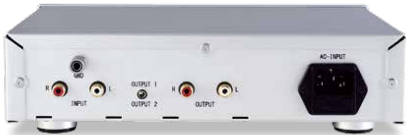
ABOVE: The DS-E3 EQ provides power for the optical pick-up's internal LEDs via the input RCAs [left]. The output RCAs [centre] offer alternative bass turnover frequencies [see Graph 1, opposite] via an 'Output 1/Output 2' toggle switch
